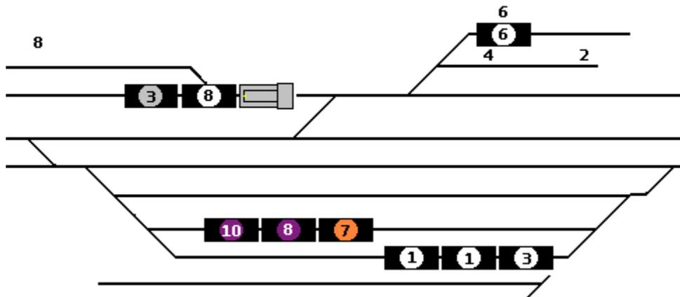
Pull the #3 car along with the #8 car out of the siding and place the #3 car on the track next to the siding. Uncouple the #8 car, and put it back on the siding next to the #8 tack.
