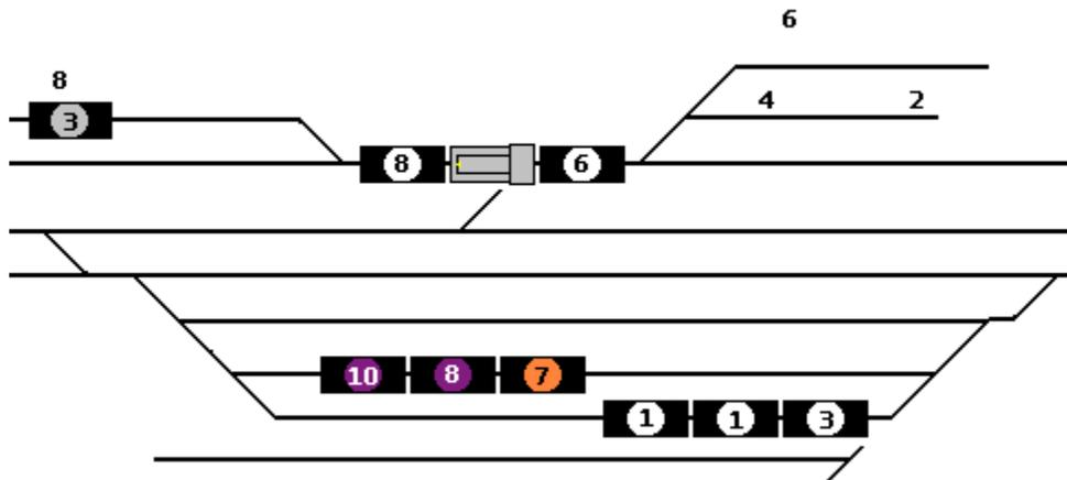
Move the engine and east cars across to the eastbound main. From here you can back up and drop off the #6 car next to the #6 tack.
